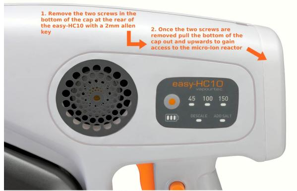
3. Once the lon covering cap has been removed pinch both sides of the reactor and pull directly outwards to remove it from the easy-HC10. Now replace it with a new one and repeat steps 1 and 2 in reverse
